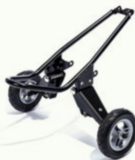
Therapy bicycle frame as assembly set for standard commercial bicycles (hub installation depth min. 120 mm)
