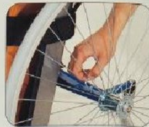
Quick-release pins allow easy removal of wheels for storage and transport.
